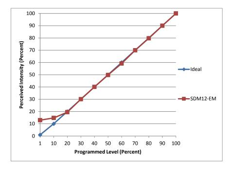
**Observations:** Mixing NDV and HDV products on a single power unit results in flick Not compatible with ScenePoint Dimmer.
